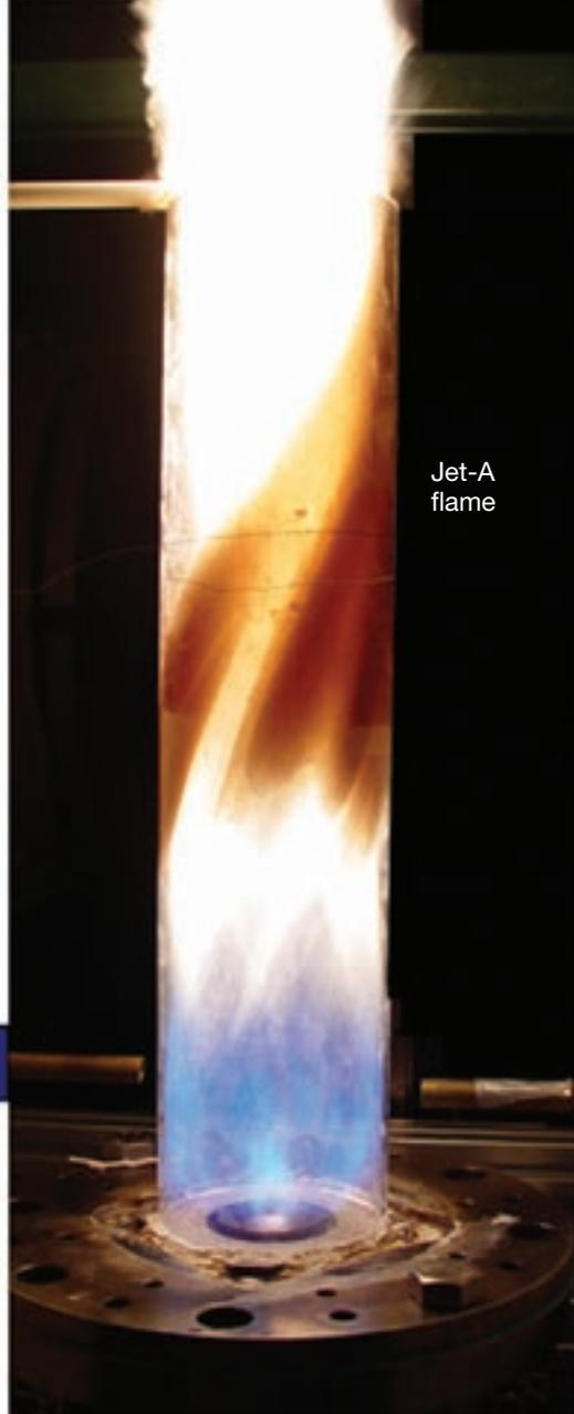
[ Diode laser based sensor in a flame fired by a realistic fuel. ]
