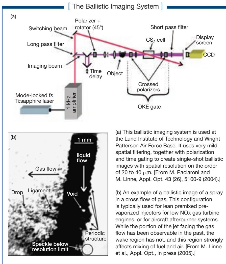
Commercially available lasers and cameras make it possible to do this twice in rapid succession, thus enabling image acceleration of these same features. Because the density of the liquid phase can be considered constant, such an image provides a two-dimensional map of the force vectors acting to tear the liquid core apart. This development can determine unambiguously the processes by which the near field breaks up.
