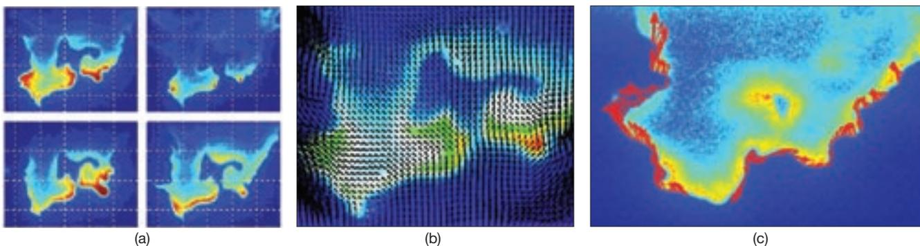
[ Rapid framing system to image dynamics of a turbulent, swirl-stabilized premixed methane air flame. This flame is related to advanced designs for gas turbine combustors, and the data have been generated for validation of detailed models. (a) Four PLIF images of OH taken in rapid succession (400  $\mu$ s time delays). (b) A simultaneous image of flow-field velocity acquired via particle image velocimetry (PIV). These data make it possible to track flame front motion (c). ]
