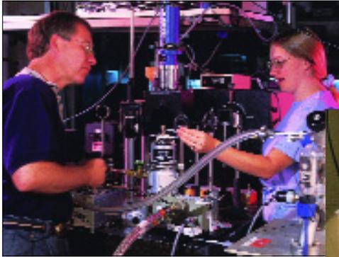
Left: Terrance Worchesky (left) works with a student to design electro-optic devices using photoluminescent measurements of quantum-well nanostructures.
