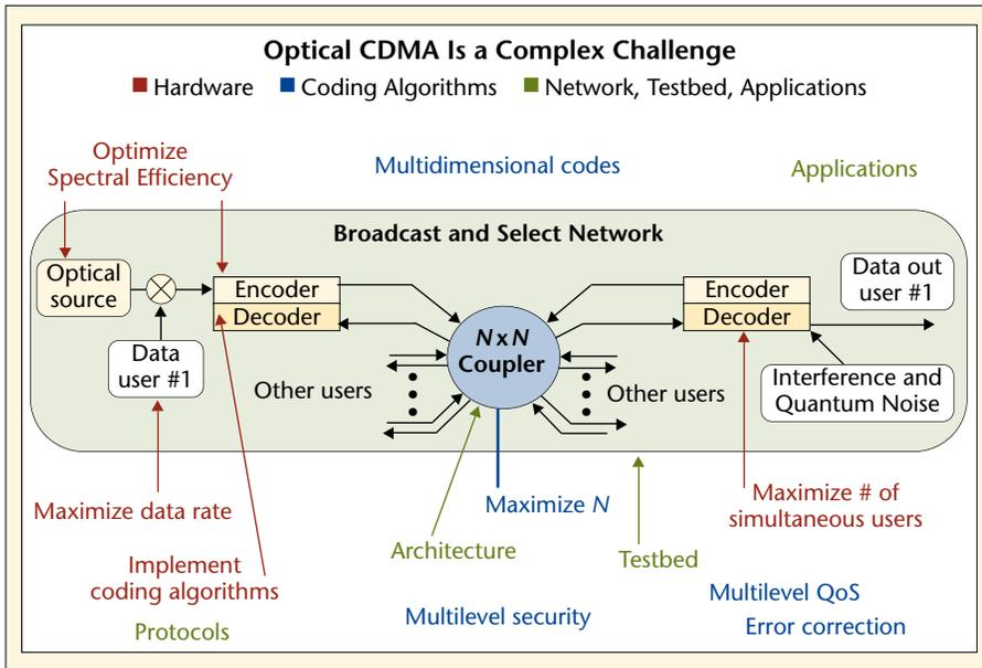
**Figure 2.** The area enclosed in the light blue box illustrates a conceptual optical CDMA network (assumed to be an  $N \times N$  star). Realization of such a network is a complex challenge based on three major components: hardware (red), coding algorithms (blue) and validation [network architecture, simulations and applications (green)].
