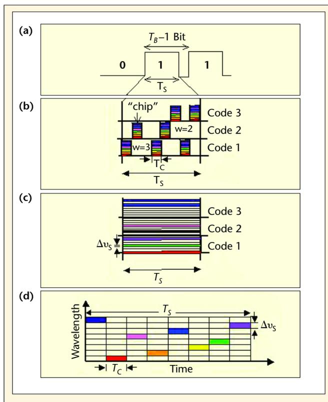
**Figure 1.** Schematic illustration of 1D and 2D optical CDMA codes. (a) Data stream; (b) 1D temporal codes, temporal chips  $T_C$ ,  $M=8$ ,  $w=2$  or 3; (c) 1D spectral codes, spectral chips  $\Delta\nu_S$ ,  $M=8$ ; (d) 2D spectral-temporal code, 8 temporal and 8 spectral chips.
