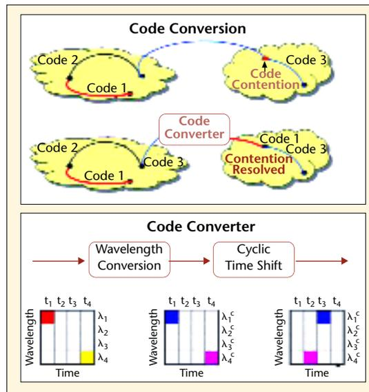
**Figure 5.** The USC team will investigate the architecture of interconnected LANs. The upper box illustrates the concept of code conversion and re-use for interconnected LANs. The lower box illustrates how wavelength conversion and time slot interchanging can be applied to code conversion.
