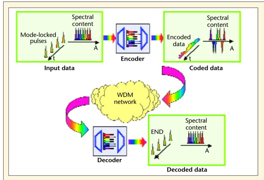
**Figure 3.** Schematic illustrating the coherent optical CDMA architecture, using mode-locked pulses as frequency bins, to be investigated by the Telcordia team.
