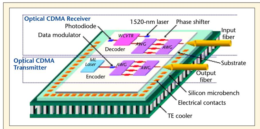
**Figure 4.** Schematic of the optical CDMA transceiver chip, packaged on a silicon-microbench platform, as proposed by the UC Davis team. (The package casing is omitted for easy viewing.) This chip incorporates advanced optoelectronic technologies including; ultrafast mode-locked lasers; arrayed-wavelength-grating multiplexers; phase modulators; and asymmetric wavelength converters. The chip dimensions are expected to be  $4 \times 4 \times 1 \text{ cm}^3$ .
