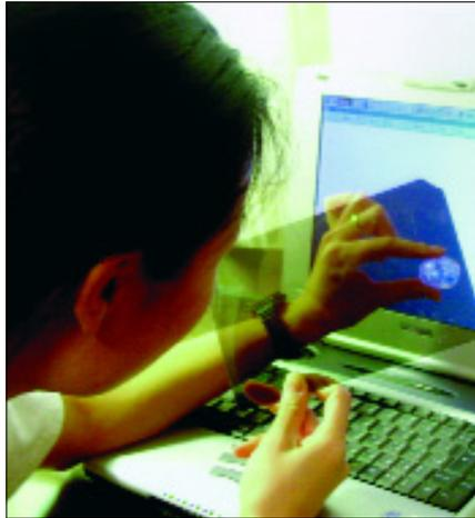
**Figure 1.** A polariscope improvised by use of the display panel of a laptop computer.
