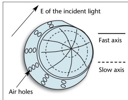
**Figure 2(a).** Cylindrically symmetric test object and its birefringence pattern. Fast and slow axes of a plastic cap.
