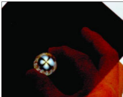
**Figure 2(b).** Birefringence pattern of a plastic cap viewed by means of the polariscope.
