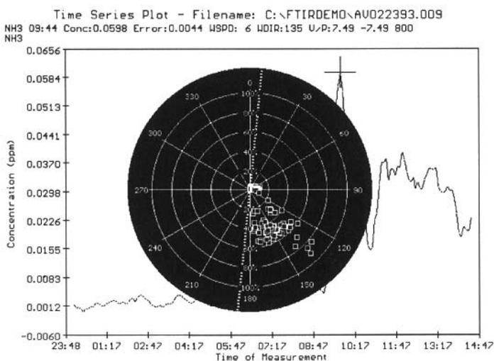
**Figure 3.** The correlation of wind direction with the observed gas concentrations of Figure 2. This plot allows the direction of the release to be detected. In this case, the emissions are coming from 150° or from the south-southeast.
