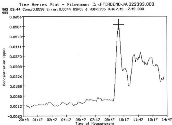
**Figure 2.** A time history plot of ammonia (NH<sub>3</sub>) at the fence line of a petrochemical facility detected by the FTIR monitoring system shown in Figure 1. The rapid increase at roughly 9:30 a.m. is a release detected by the system. The cross hair at the peak shows the concentration (0.059 ppm) and error ( $\pm 0.004$  ppm) listed at the top of the plot.
