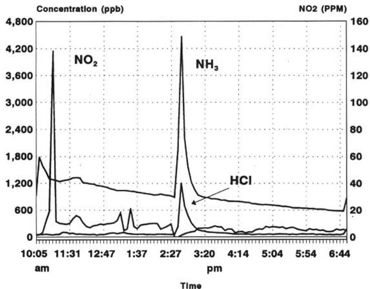
**Figure 5.** A time history plot of gas concentration observed in a semiconductor scrubber exhaust. The spikes of NO<sub>2</sub>, NH<sub>3</sub>, and HCl are correlated with activities of the batch manufacturing process. Real-time monitoring of these and other acid gases is a powerful capability of FTIR.
