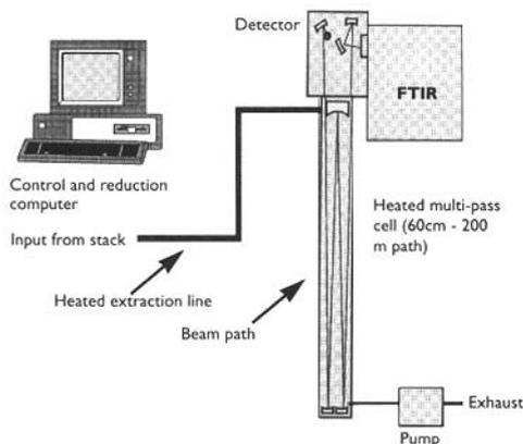
**Figure 4.** Schematic of an extractive FTIR monitor as used for stack monitoring. Heated input and output lines are used and the multipass cell provides long path-lengths by re-imaging the IR light repeatedly before allowing it to exit. Cells from 4 m to over 100 m are commercially available.
