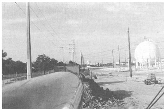
**Figure 1.** Photograph of the beam path for a fence-line FTIR monitoring system operated by Radian Corp. at a petrochemical plant in Houston, Texas. The plant is to the right and the residential area to the left. The prevailing wind is off the plant and into the residential area.
