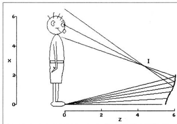
Figure 2. Concave cylindrical mirror ray trace
