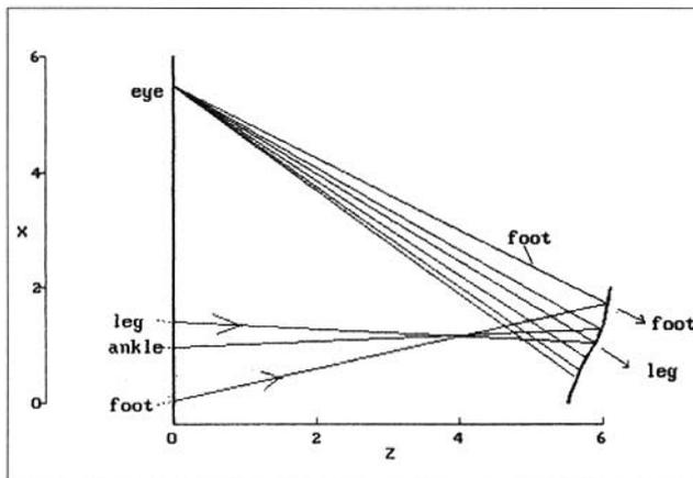
**Figure 4. Ray trace to eye from foot and leg: Concave cylindrical mirror**
