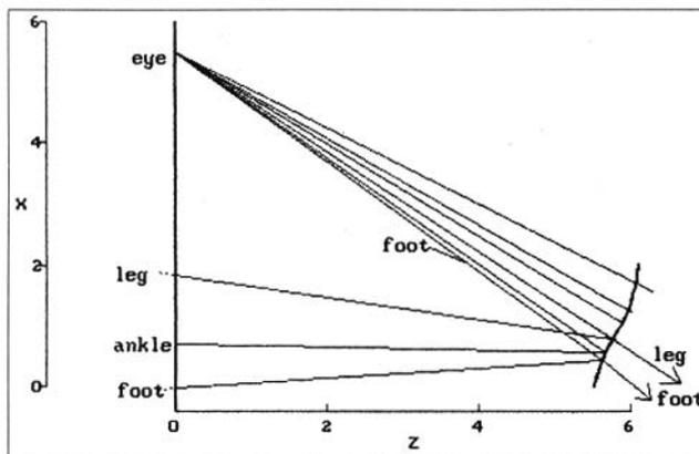
**Figure 3. Ray trace to eye from foot and leg: Convex cylindrical mirror**
