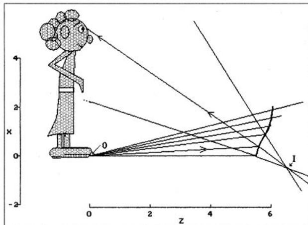
Figure 1. Convex cylindrical mirror ray trace
