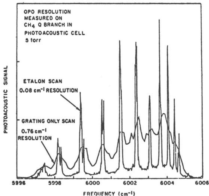
Grating-only ( $0.76\text{-cm}^{-1}$  resolution) and grating-plus-etalon ( $0.08\text{-cm}^{-1}$  resolution) photoacoustic spectral scans of the  $\text{CH}_4$  overtone  $Q$ -branch spectrum at 5-Torr pressure, taken using a computer-controlled  $\text{LiNbO}_3$  OPO at Stanford University by Martin Endemann and Robert Byer. The OPO has a  $4500\text{-cm}^{-1}$  tuning range.
