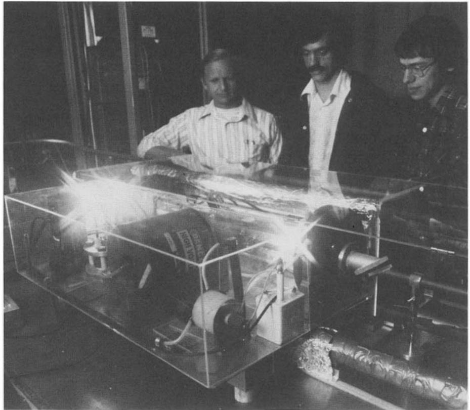
Single-longitudinal-mode TEA  $\text{CO}_2$  laser used at Texas Tech University to obtain narrow-linewidth, high-power output with precision and accuracy comparable with that of a narrow-band-diode laser. Left to right, Martin Gundersen, Terry Yocom, and Roger Dougal.
