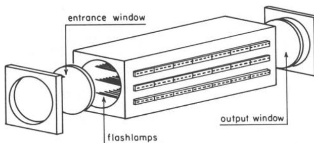
Flashlamp-pumped iodine amplifier envisaged as part of an eight-beam laser structure at Laboratoire de Marcoussis in France. Flashlamps are in the gain medium.
