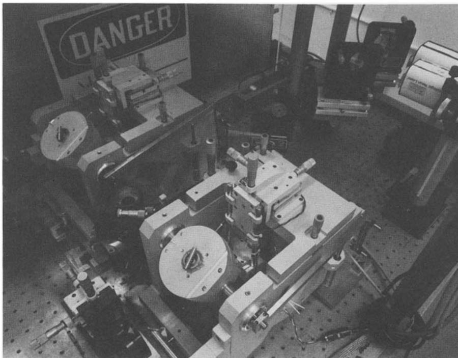
Cadmium selenide OPO used at Los Alamos Scientific Laboratory for 16- $\mu\text{m}$  generation. The OPO is pumped by an HF laser. The work was reported by Robert Wenzel and George Arnold.
