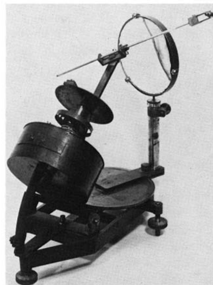
Fig. 4. Heliostat used by Michelson to focus scan light on the entrance slit for the first velocity-of-light experiment. The heliostat was borrowed by Michelson from the Army Medical Museum.
