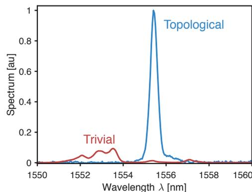
Left: Top-view photograph of the lasing pattern (topological edge mode) in a  $10 \times 10$  array of topologically connected resonators, and the output ports. Center: Output intensity versus pump intensity for a topological-insulator laser and its corresponding trivial counterpart. The enhancement of the slope efficiency is approximately threefold. Right: Emission spectra from a topological-insulator laser and its topologically trivial counterpart.
