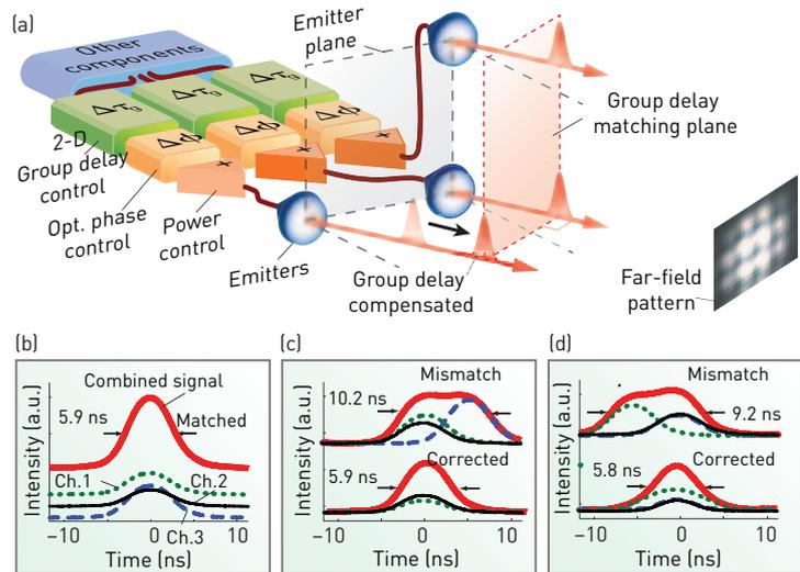
(a) A SLIDAR system capable of 2-D beam steering; normalized time traces of the returned signal when the system is (b) pointing on-axis, (c) tilted in the  $x$  direction, and (d) tilted in both the  $x$  and  $y$  directions. The thick red line is the combined signal, while the thin lines are the signal from three individual channels.
