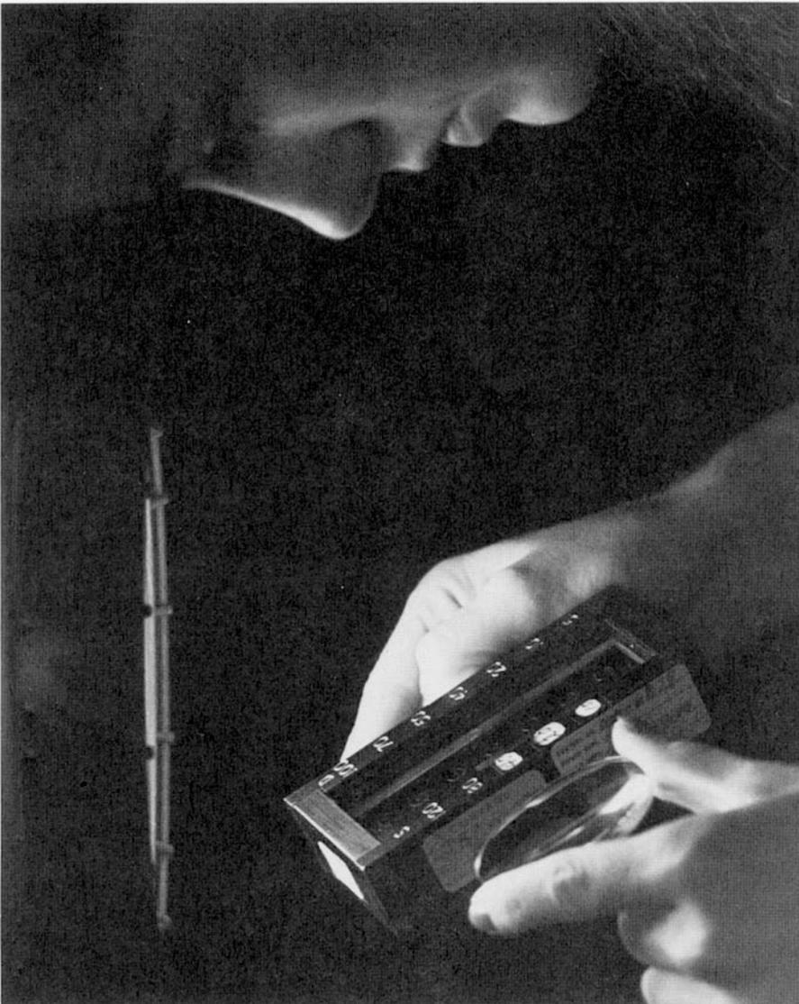
Scratch-and-dig defects on a lens surface compared with calibrated standards.
