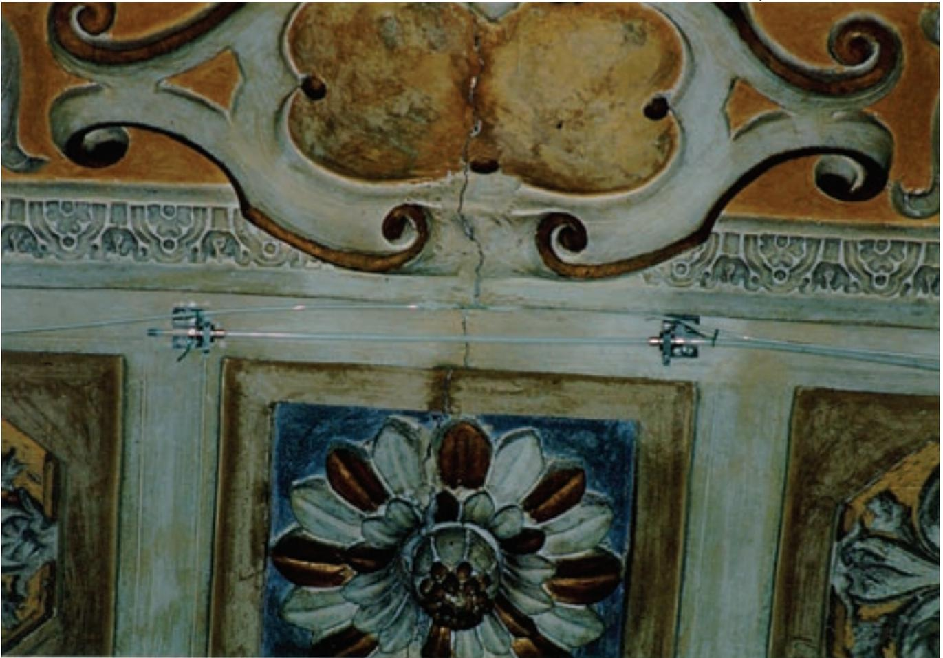
The SOFO displacement center shown here monitoring crack development in the 17<sup>th</sup> century Gandria Church in Switzerland.
