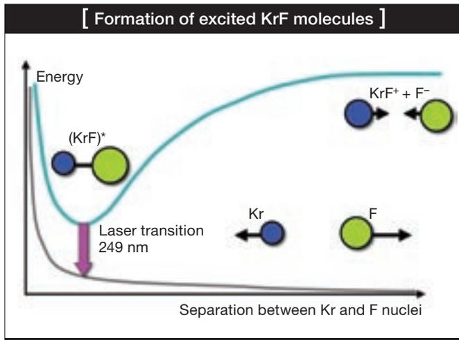
The main reason why the RGH lasers and CO<sub>2</sub> differ so much in their division of labor between sustaining the ionization rate and exciting the upper laser level precursor species is that the energy required to create the Kr<sup>+</sup> ions needed for reaction (2) is the same or very close to that required for creating electron-ion pairs to sustain the discharge.
