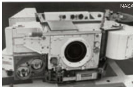
(Top) Apollo 15 command module *Endeavour*, in a photo taken from the lunar module Falcon in lunar orbit, shows the instrument bay containing the lunar mapping camera and ruby lidar. (Bottom) The Apollo lunar mapping camera on a lab bench prior to flight. The lidar occupies the lower left portion of the instrument.
