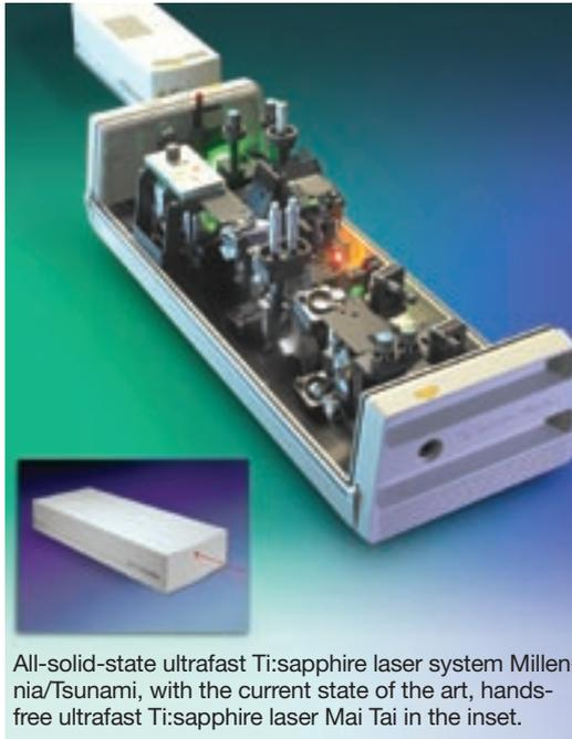
All-solid-state ultrafast Ti:sapphire laser system Millennia/Tsunami, with the current state of the art, hands-free ultrafast Ti:sapphire laser Mai Tai in the inset.
