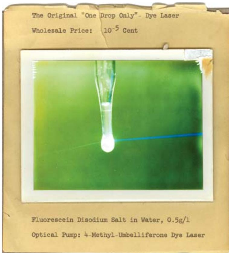
"One-Drop-Only" dye laser, a precursor of the edible laser. This picture was posted on a laboratory door at Stanford in 1970.
